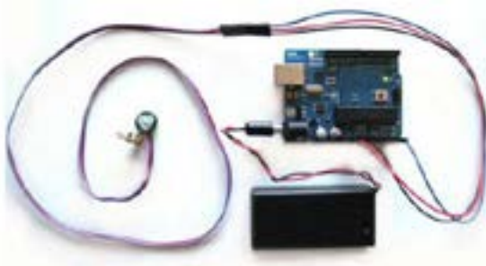
Fig. 3. Heart Pulse Sensor. Source: https://pulsesensor.files.wordpress.com/2011/09/arduino-plug-in3.png?w=460&h=345
